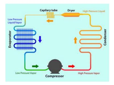
The compressor compresses the refrigerant, causing it to become a hot, high pressure gas (red in the diagram).
